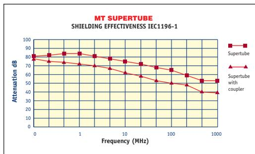
The graphs above show that the shielding effectiveness of MT Supertube is highly effective throughout the entire frequency range and will provide protection from interference for data, telecoms and signal cables.
